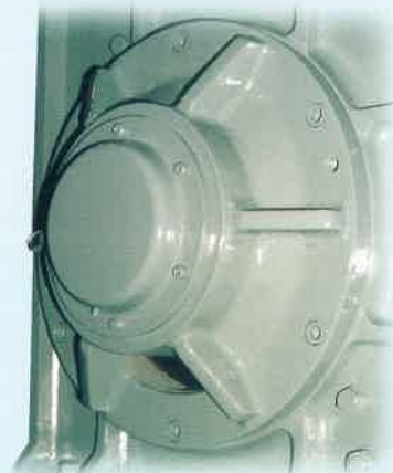
粉砕機軸受の理想形“セミアウトサイド式” Semi-Outside Type, an ideal granulator bearing
