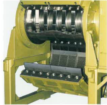
スクリーン受け開放時 Machine with screen supporter opened
